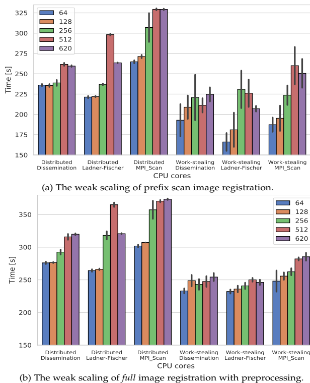
Fig. 11: The weak scaling of image registration on Ivy Bridge. Figures begin at value 150 for better readability.
